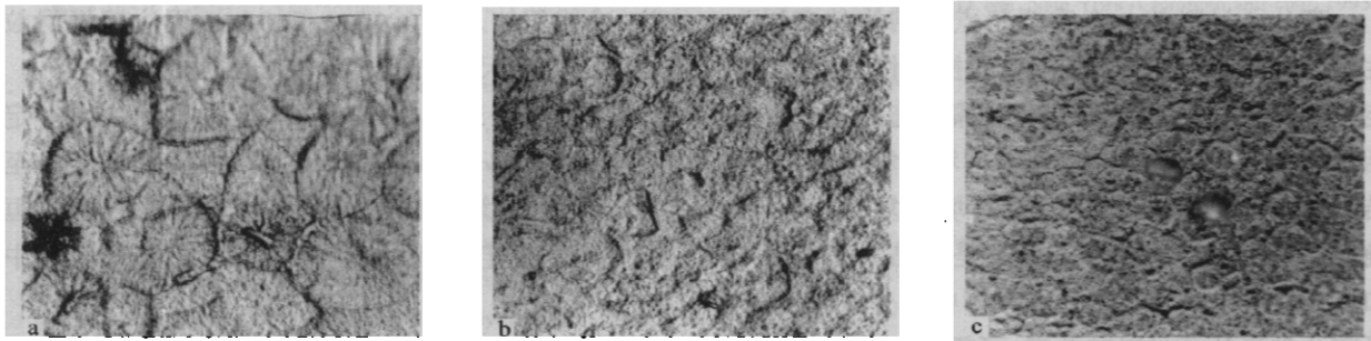
Fig. 1 The microscope photos of PP with different filled quantity of nucleating agent( \times 500 )
